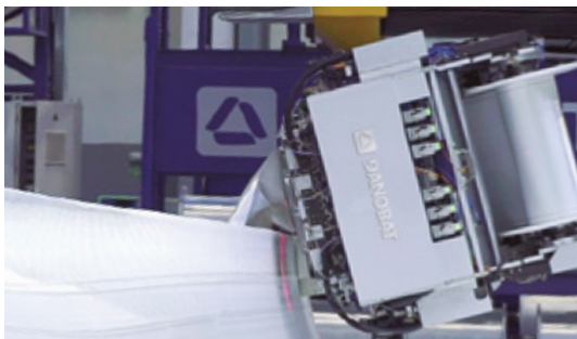
▲ Cutting on the fly & Selective application of binder/tackifier
